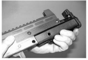
(5) Remove upper receiver from lower receiver.
