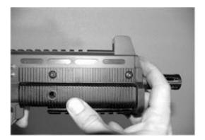
(7) Push retaining pin through right side until fully seated.
