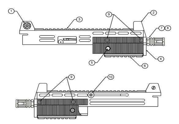
1 Insure firearm is unloaded. Point in a safe direction. Remove magazine and pull bolt to the rear to insure chamber is empty.
